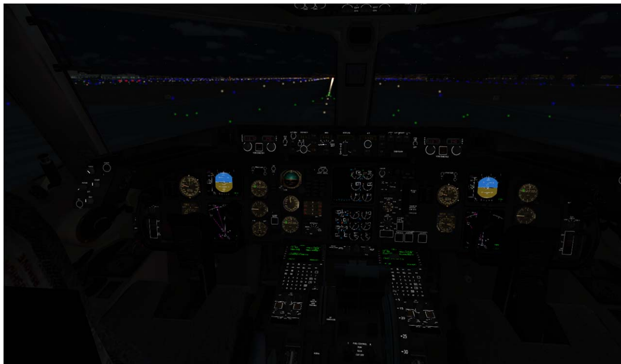
Text Backlighting with flood lighting Off
